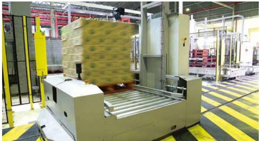
An automatic palletising solution at the Coca Cola’s Cikedokan plant comprises layer-by-layer palletisers, pallet conveyors and a stretch wrapper to cover the loaded pallets
